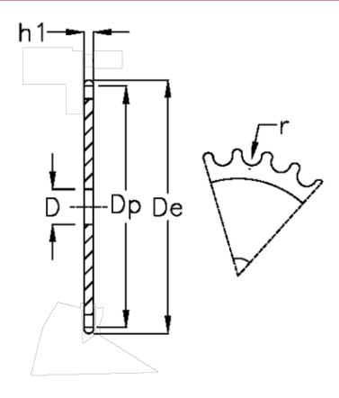
C = 5 D = 25 De = 148.4 Dp = 129.96 For chain size = 1  $3/4 \times 1 1/4$ For chain type = 28 B-1 h1 = 29.4
